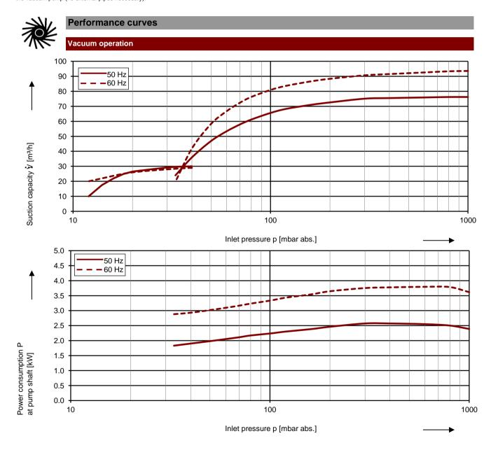
The characteristic curves are based on the evacuation of 100 % saturated air and an intake temperature of 20 °C. At a suction pressure of 1013 mbar abs. and a temperature of the operating liquid of 15 °C (water as operating liquid) the characteristic curves will be achieved. The tolerance is  $\pm$  10 %.
